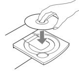
• Make sure the disc is centered in the tray in order to avoid any malfunction or jamming of the tray or damage to the disc itself.
